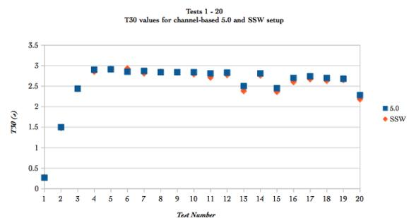
Figure 17: T30 results for all 20 measurements at mic position 1 for 5.0 setup (blue) and SSW setup (orange).
