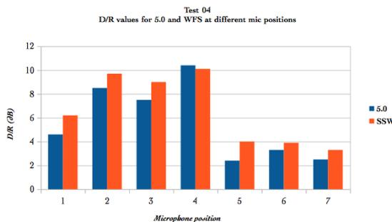
Figure 10: DRR values for test 4 from 5.0 setup (blue) and SSW setup (orange) at the 7 different mic positions.
