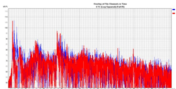
Figure 8: ETC for test 13 from 5.0 setup (red) and SSW setup (blue).
