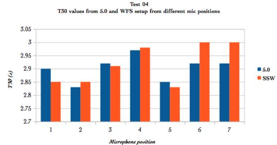
Figure 11: T30 values for test 4 from 5.0 setup (blue) and SSW setup (orange) at the 7 different mic positions.
