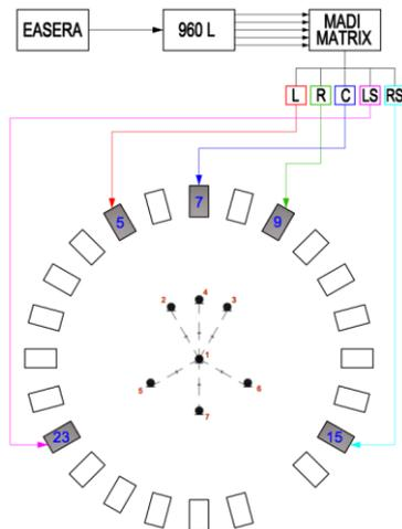
Figure 1: Loudspeaker array with chosen microphone positions for RIR measurements of the channel-based 5.1 system.
