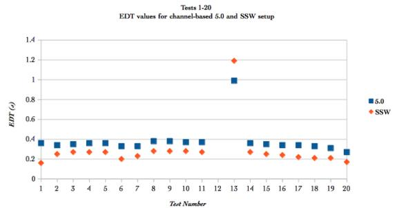
Figure 15: EDT results for all 20 measurements at mic position 1 for 5.0 setup (blue) and SSW setup (orange).
