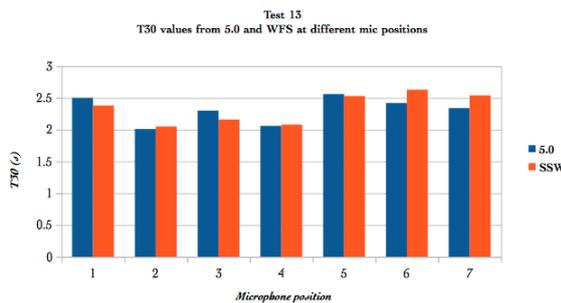
Figure 14: T30 values for test 13 from 5.0 setup (blue) and SSW setup (orange) at the 7 different mic positions.
