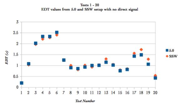
Figure 16: EDT results without direct signal for all 20 measurements at mic position 1 for 5.0 setup (blue) and SSW setup (orange).
